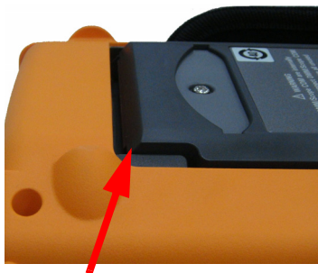
Figure 8-1 Push towards the arrow direction to remove the stand
