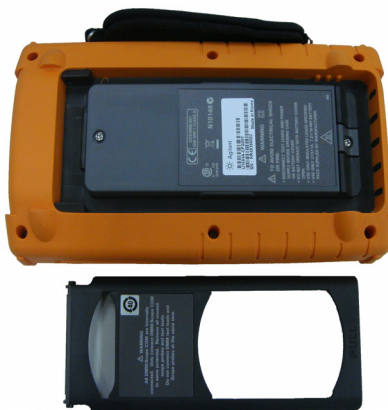
Figure 8-2 Disassemble the stand from the instrument
