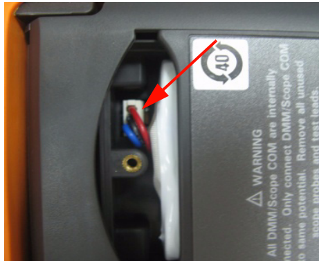
Figure 8-6 Unplug 2-wire connector with a tweezers.
