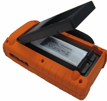
Figure 8-5 Remove battery pack cover without removing stand
