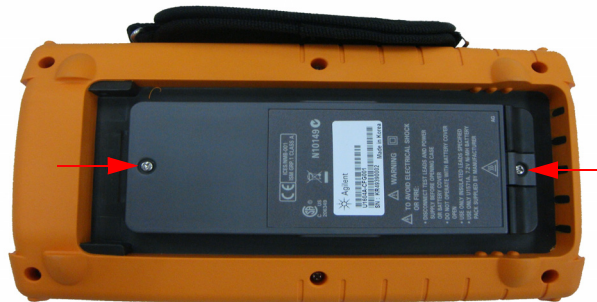
Figure 8-3 Remove battery cover screw
