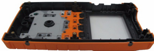
Figure 8-12 Remove keypad from the front cover
